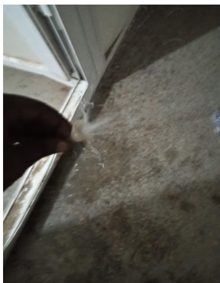
Fig. 10: The sprinkler if there is LPG detection
