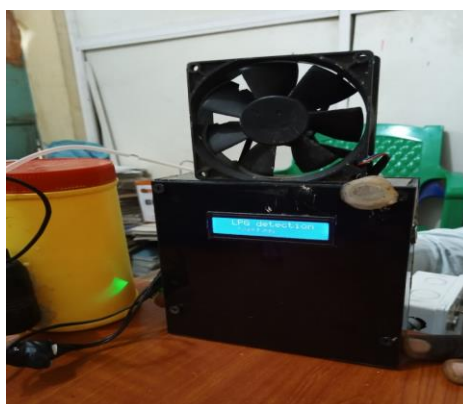
Fig. 2: LPG detection system implementation result
