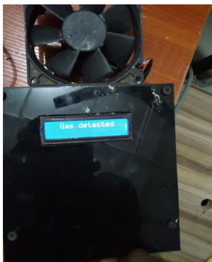
Fig. 5: The implementation result shows there is LPG present in the environment
