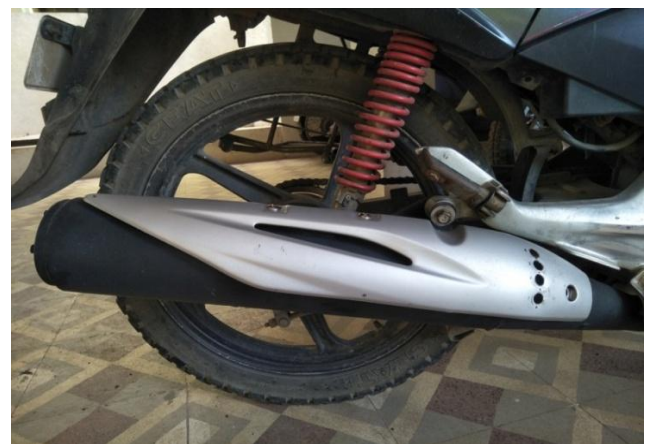
Fig3 Muffler Guard Cut At Big End With 4 Vertical Holes (Case 1)
