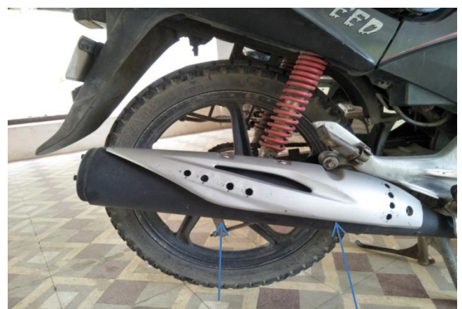
Fig4 Muffler Guard Cut At Big End With 4 Vertical and 4 Horizontal Holes (Case 1)
