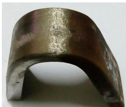
Fig 7 Face bent of weld joint
