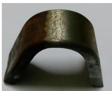
Fig 8 Root bend of weld joint
