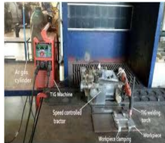
Figure 3: Automated TIG welding setup
