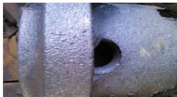
Figure 2. Sand Inclusion defect in Transmission Case casting
